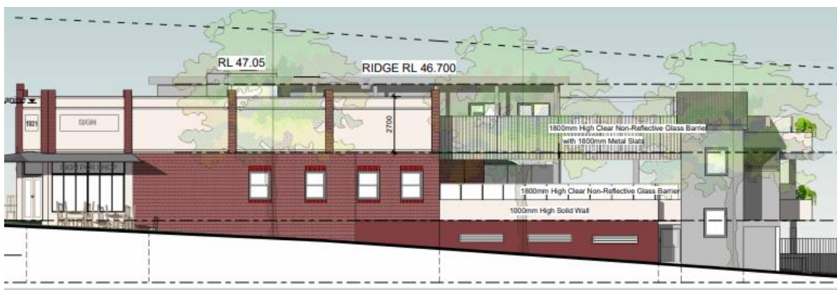
Figure 21 - Southern Elevation Plan depicting the appearance of the previous proposal from Arthur Street with an FSR of 1.49:1
