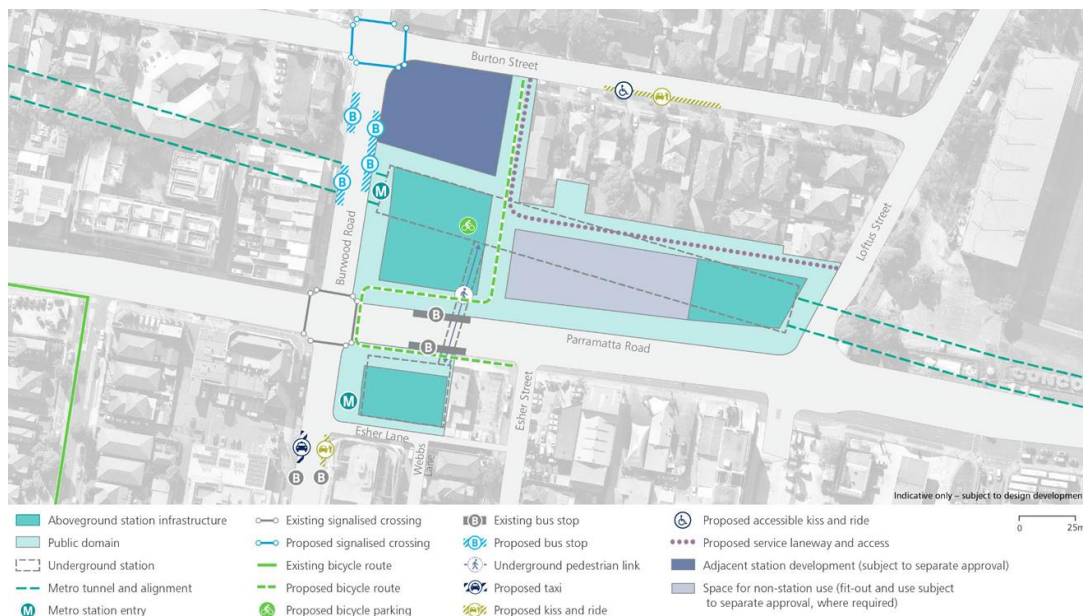
Figure 10 Proposed Burwood North Metro Station arrangement
