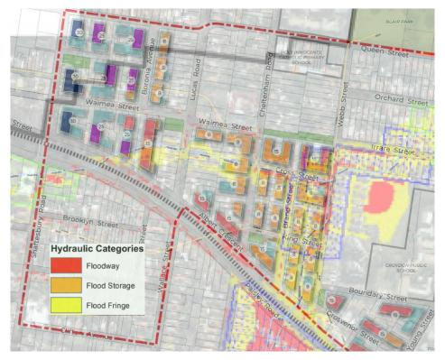
Figure 12: 1% AEP Flood Hydraulic Categories and Flood Hazard and Emergency Response Classifications (blue-dotted area = Low Flood Island)
