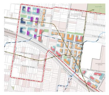
Figure 1: Sydney Water sewer (dark brown) and stormwater (blue) assets within the Master Plan area
