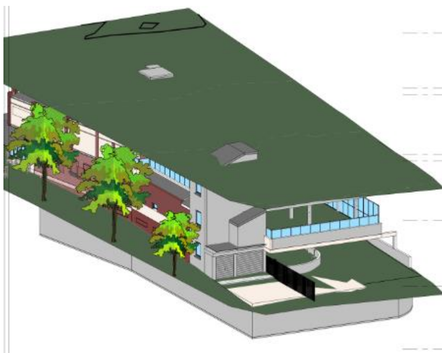
Figure 15 – Extract of applicant's 3D photomontages showing the extent of the lift overrun and fire stairs above the 10m height limit
